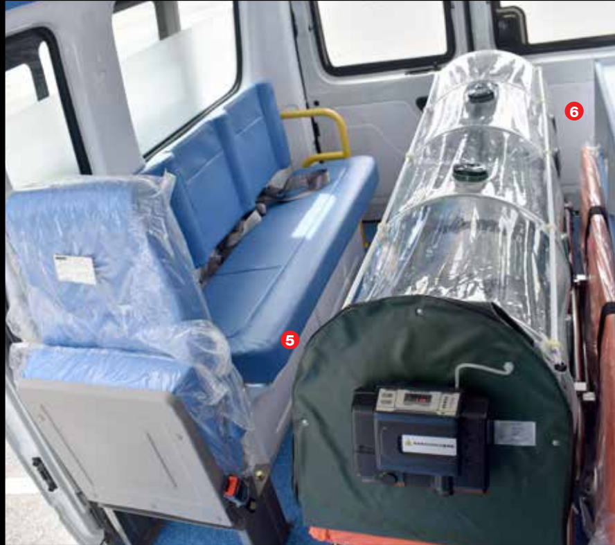
5 Isolation Pod 6 Cabinet & Electrical Power Points
