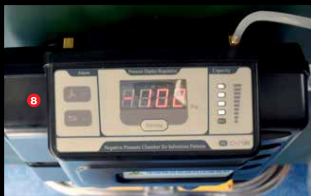
7 Bright Interior Lights & UV Sterilizer Lamps 8 Isolation Pod Electronic-Control Negative Pressure
